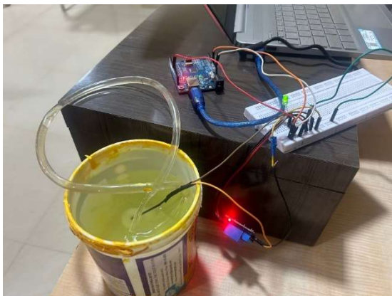
Fig 2. The hardware implementation of smart water pumping system with customized time period irrigation system.
